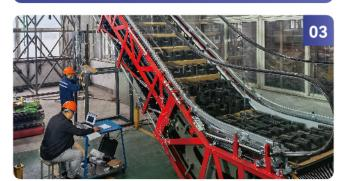
EME在工厂内完成装配后,进行静载试验,其桡度已符合标准。 After completing assembly in the factory, EME conducted a static load
